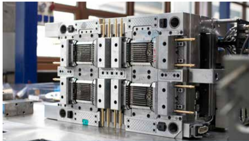
Half of a finished mould before the final acceptance test in the factory
